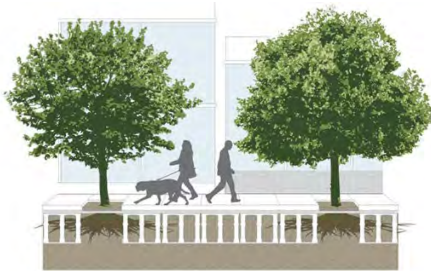
Image: Suspended pavement system.
